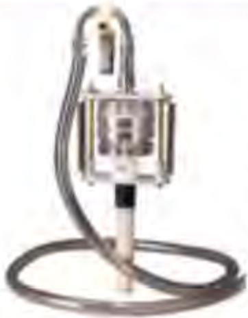
10 mm nylon cyclone is used in NIOSH & OSHA sampling methods.
