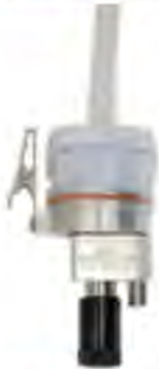
HD style cyclone with US style cassette is specified in numerous NIOSH protocols
